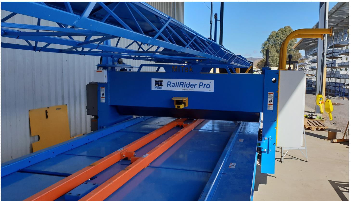
The RailRider™ floor truss roller press, along with our RailRider™ Pro tables provides the ultimate in quality and convenience - and all the features needed for high production and safe, reliable performance! The system can be customised with different table lengths available, configurable pneumatic setups and preset camber can be applied.
